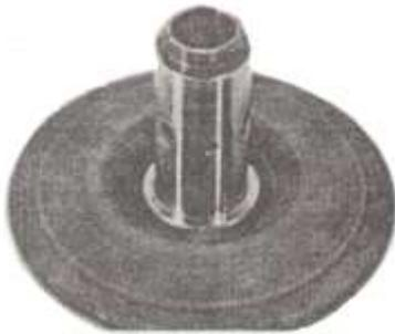
20. Check secondary sliding sheave wear.
