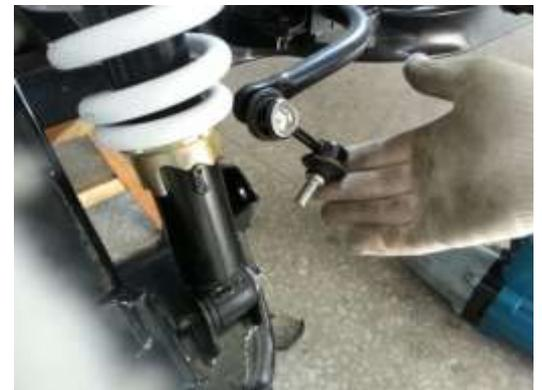
4. Remove the two bolts that secure the stabilizer bar to the main frame, each side.
