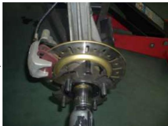
7. Rotate hub. It should rotate smoothly without binding or rough spots or side play.
