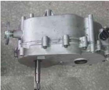
2. Remove transmission case fixing bolts.
