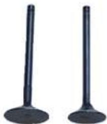
12. Check valve stem bend and check for burnout. Clean carbon deposits off its surface.
