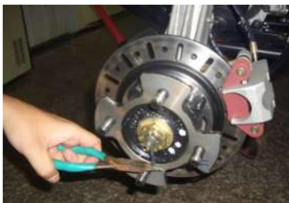
7. Rotate each bearing by hand and check for smooth rotation. Visually inspect bearing for moisture, dirt, or corrosion, or roughness is evident.
