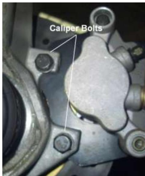
3. Remove the two caliper bolts and caliper from mounting bracket.
