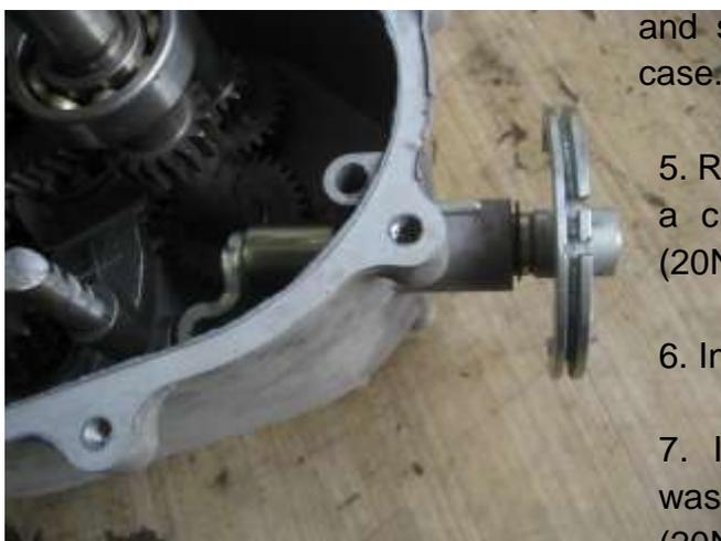
5. Reinstall left crankcase and torque bolts in a cross pattern in 3 step to 14.5 ft.lbs. (20N • m).
