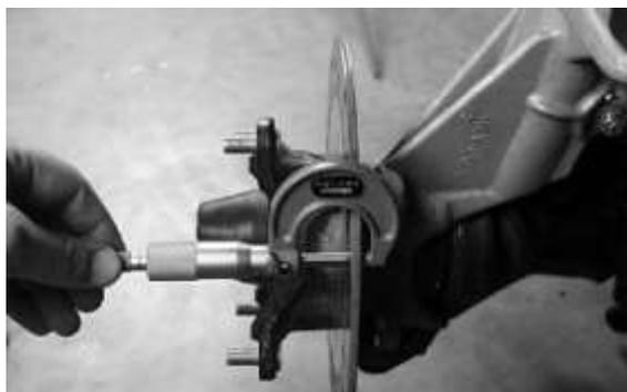
2. Measure the disc thickness at 8 different points around the pad contact surface using a 0-1" micrometer and a dial indicator. Replace disc if worn beyond service limit.
