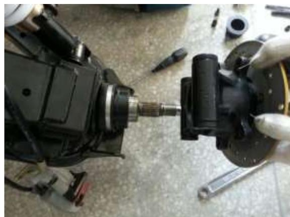
3. Pull the rear drive axle straight out of the frame. Use short sharp jerks to free the circlip from the gearcase. The circlip holds the axle in the gearcase.
