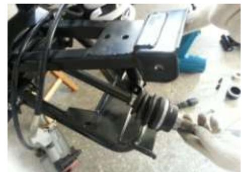
7. Loosen the bolt that secure the A-arm to frame by alternating each about 1/3 of the way until A-arm can be removed. Perform this procedure on the upper A-arm.
