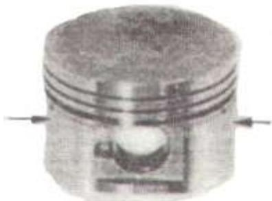
8. Measure piston outside diameter from an angle of 90° to piston pin bore, in a position some 9mm from piston bottom.
