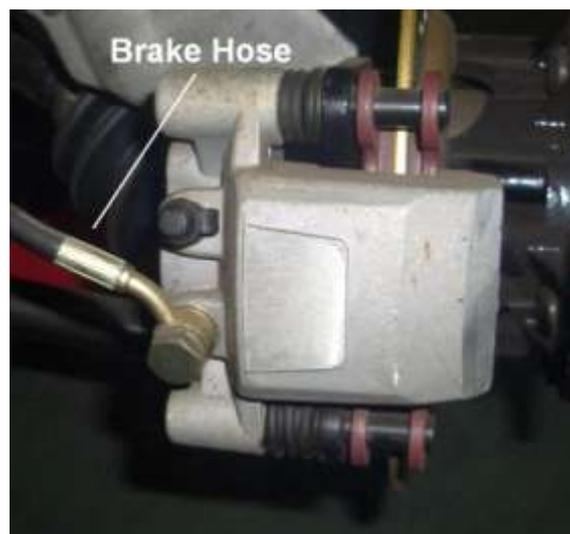
1. Remove wheel, remove caliper from the strut.
