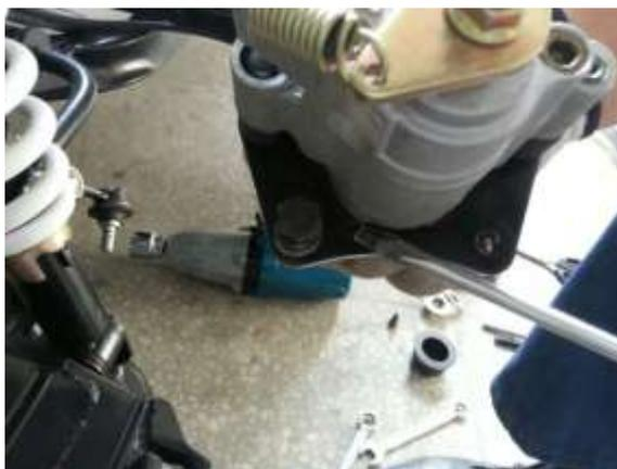
2. Measure the thickness of the caliper parking brake pads. Replace pads if worn beyond the service limit.
