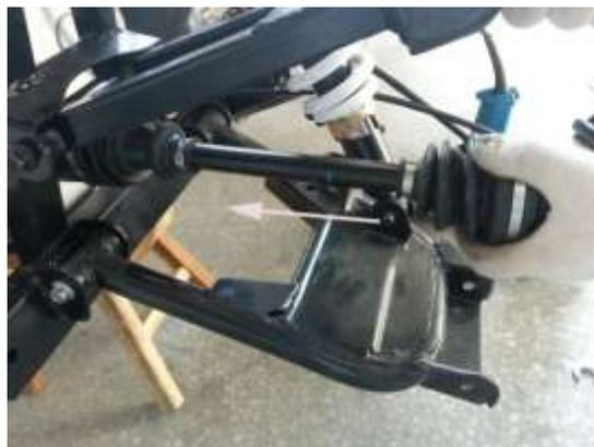
3. Slide the rear drive axle into the knuckle.
