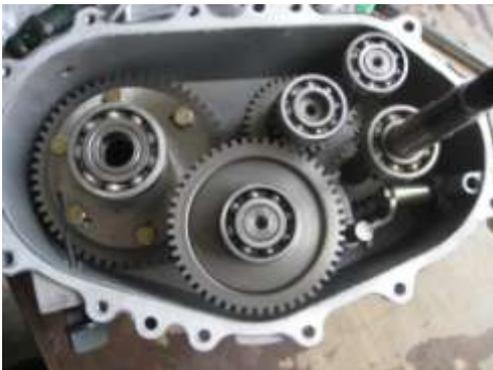
3. Knock the input shaft carefully with a soft face hammer to separate the transmission case from the left crankcase.
