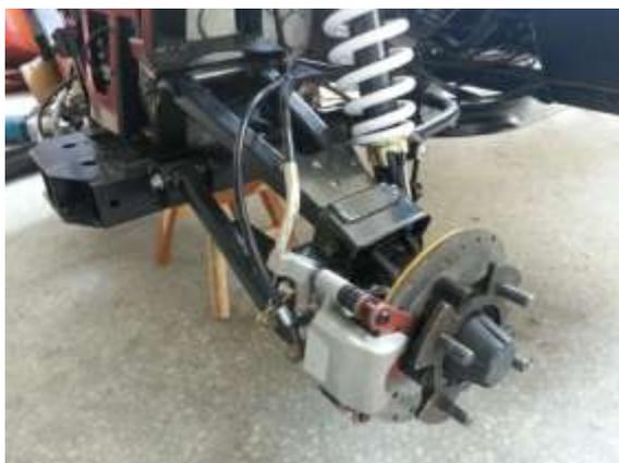
2. Inspect the parking brake cable at the parking brake lever assembly on the brake caliper.
