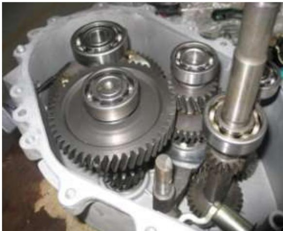
4. Prior to reinstalling the transmission make sure the mating surfaces are clean and dry, and shafts are fully seated in transmission case. Apply silicon glue to mating surfaces.
