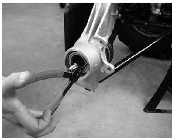
2. From the back side, tap on the outer bearing race with a drift punch in the reliefs as shown.
