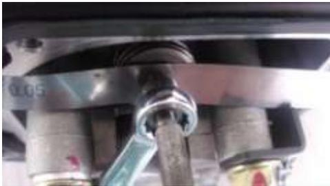
2. Rotate cooling fan to set the mark on camshaft sprocket in Top Dead Center position, that is, to align the timing line on the rotor with the mark on the crankcase.
